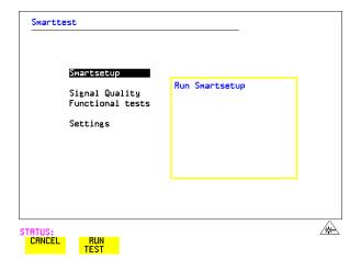
3 With Smartsetup highlighted, press **RUN TEST** to auto-discover information about the receive signal. Or press **CANCEL** to exit Smart Tests.
